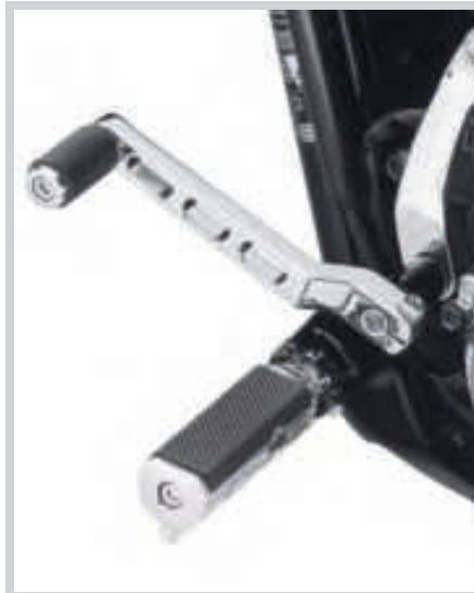
B. BILLET STYLE REAR SHIFT LEVER – FORWARD CONTROLS – CHROME
