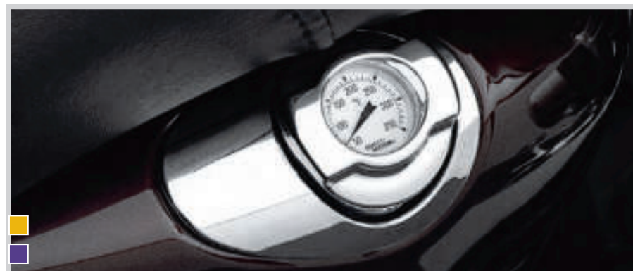
B. OIL DIPSTICK WITH TEMPERATURE GAUGE ('04-LATER SPORTSTER SHOWN)
