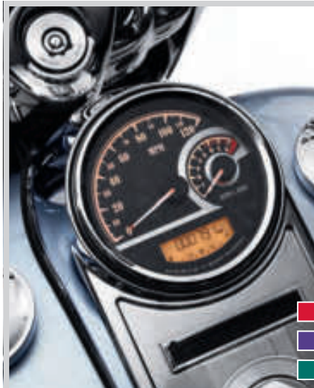
H. COMBINATION ANALOG SPEEDOMETER/TACHOMETER – 5" BLACK DIAL
